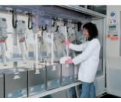
Technology that makes quality possible: Ultrasonic cleaning of quartz blanks for perfect surfaces.
