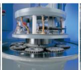
Grinding of quartz blanks: The right surface for the right frequency.
